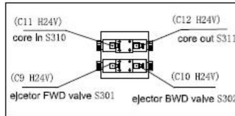
core ejector manifold
